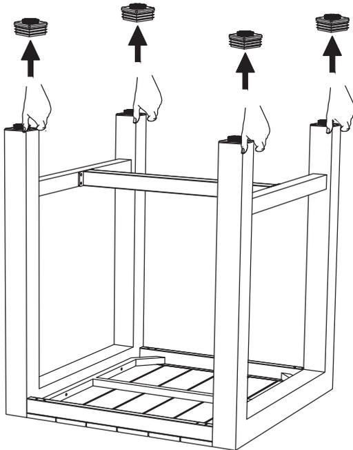
**Step 2** Lock the brake on each castor. Screw each castor into the bracket inside the leg.
