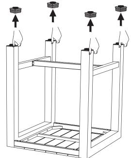
Step 2 Lock the brake on each castor. Screw each castor into the bracket inside the leg.
