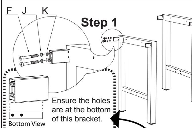
Ensure the holes are at the bottom of this bracket.
