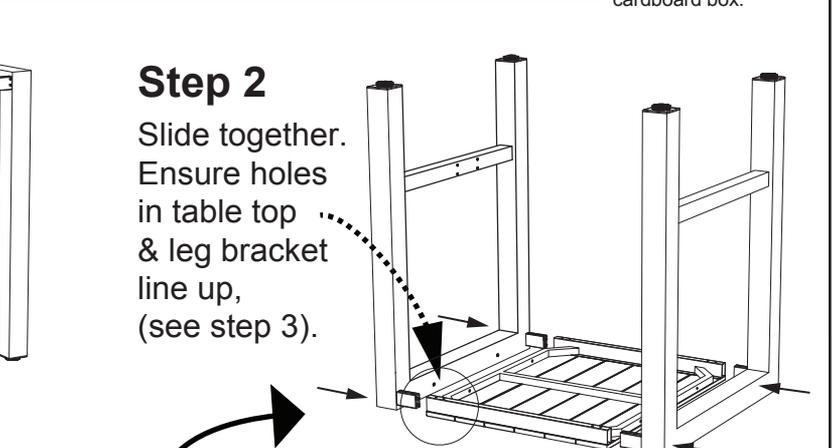
**PLEASE NOTE:** you only need to hand tighten this bracket. You may need to loosen one bracket if the table top does not slide smoothly into place. (These do not need to be tightened further.)
